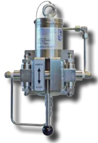
The Sentry® Magnetic Trap isolates magnetite particulates to protect both sample conditioning and analytical instrumentation from critical down time and costly repairs. The Magnetic Trap uses high strength neodymium magnets that are inserted into the core of the trap to attract and capture magnetite.
